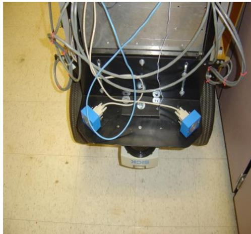
**Figure 3: Ultrasonic transducers (blue boxes)**
