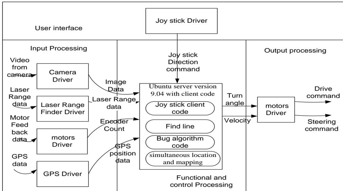
Figure 7: Software Architecture Context Diagram
